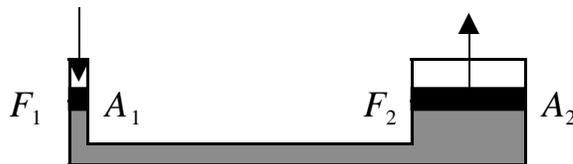
If the area  $A_2$  is much larger than the area  $A_1$ , then a small force  $F_1$  can be applied to create a large force  $F_2$  at the output end. This large force can be used to jack up a car or lift heavy objects.
