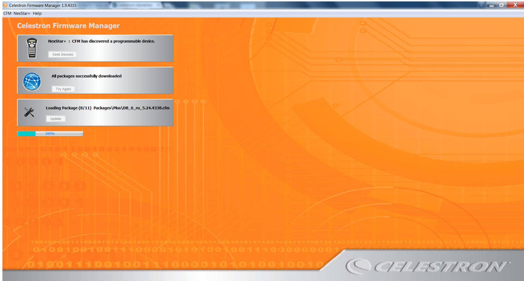
When it finishes, a popup may come up stating it's done and after clicking ok, it should look like this. Exit the program. Turn off the telescope. Unplug the RS 232 cable from the controller, and turn it back on to check that it loads properly.
