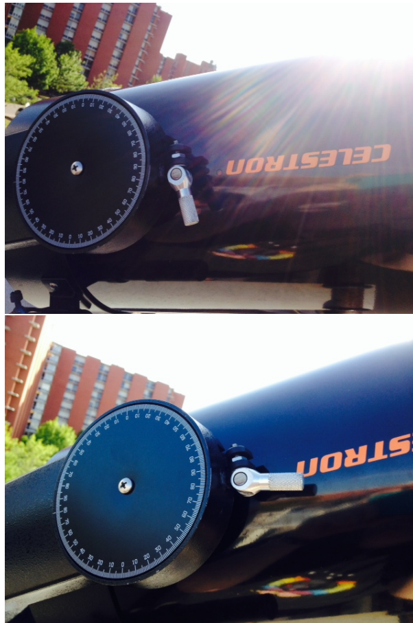
Figure 5: Declination brake. Can unlock the brake so that it is parallel to the mechanism it rests on, seen in the top picture. Twist the knob and lock the brake in place (perpendicular to the mechanism, seen in bottom picture) so that the brake has a tighter hold on the telescope.
