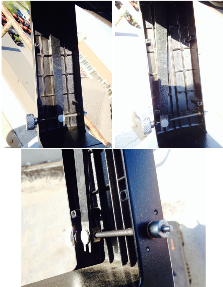
Figure 2: Upper left shows center (best) configuration of declination arm, the central bar seen in the picture. Upper right shows the arm against one side. If you keep turning the declination knob in the same direction, the smaller knob and bushing shown in the bottom picture can pop off the other end and be nigh impossible to find in the dark. Also the forks on the end of the declination arm can break, causing the declination adjustment to be unusable. To avoid this, center the arm before class/ event.
