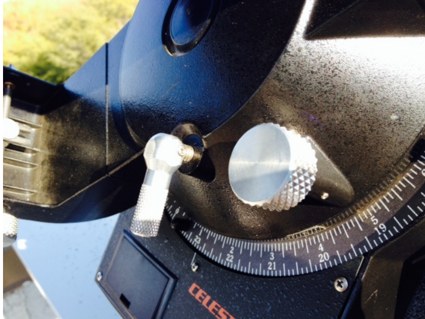
Figure 1: 2 of the knobs that can be loose so that turning them achieves nothing. There is the RA brake (the silver L-shaped one) and the RA fine adjustment knob (silver wide cylinder) On the L-shaped one, you can see at the corner of the L is the set screw that can be tightened. The other knob has a set screw that can be seen on its base.
