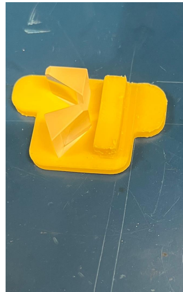
3D printed prism mount
