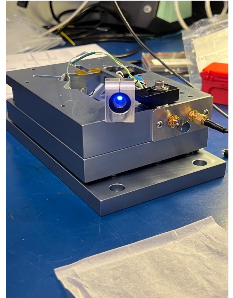
Laser diode installed
