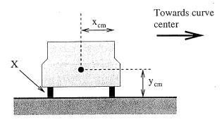
When the car is at rest, the center of mass of the car is located at a point  $y_{cm}$  above the road and a distance  $x_{cm}$  from either wheel. Treat the wheels as having a negligible width.
