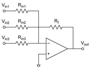
$$V_{out} = A_{V1}V_{in1} + A_{V2}V_{in2} + A_{V3}V_{in3} + \cdots$$
