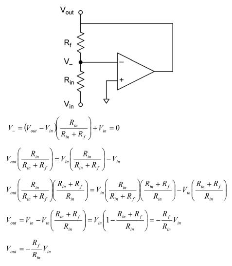
The input impedance of the inverting amplifier is determined by  $R_{\rm in}$ . Note that  $V_-$  is held at the same voltage as  $V_+$  by the op amp feedback. Because  $V_+$  is connected to ground, the input impedance is just  $R_{\rm in}$ .
