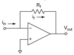
$$\begin{aligned} V_{out} &= -R_f I_{in} \\ A_Z &= \frac{V_{out}}{I_{in}} = -R_f \\ \frac{\mathrm{d}\, V_{in}}{\mathrm{d}\, I_{in}} &= 0 \end{aligned}$$
