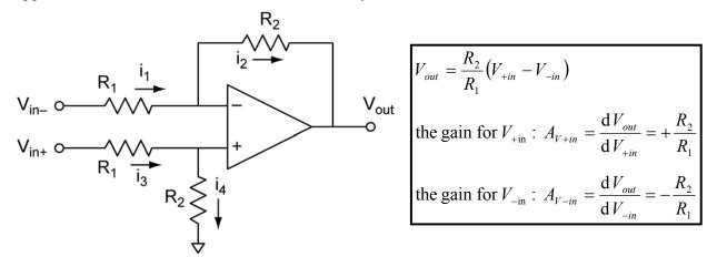
Analysis of the differential amplifier starts with our op amp golden rules. From rule #4 we know that  $V_- = V_+$ . From rule #3 we know that  $I_1 = I_2$  and that  $I_3 = I_4$  because no current flows into the inputs.
