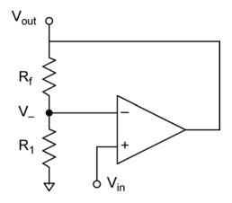
$$\begin{split} V_{-} &= V_{out} \Biggl(\frac{R_1}{R_1 + R_f}\Biggr) = V_{in} \\ V_{out} \Biggl(\frac{R_1}{R_1 + R_f}\Biggr) \Biggl(\frac{R_1 + R_f}{R_1}\Biggr) &= V_{in} \Biggl(\frac{R_1 + R_f}{R_1}\Biggr) = V_{in} \Biggl(1 + \frac{R_f}{R_1}\Biggr) \\ V_{out} &= V_{in} \Biggl(1 + \frac{R_f}{R_1}\Biggr) \end{split}$$
