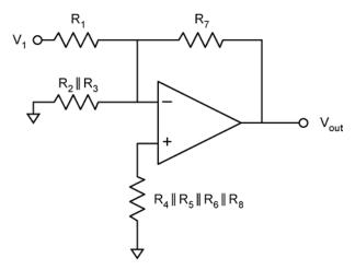
Notice that the non-inverting input,  $V_+$  is connected to ground though a resistor. Because no current flows into the op amp's inputs,  $V_+ = 0$ , equivalent to it being connected directly to ground (see below).
