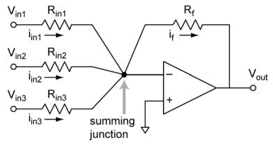
Analysis of the summing amplifier starts with our op amp golden rules. From rule #4 we know that  $V_- = V_+$  and that  $V_- = 0$  because  $V_+$  is connected to ground. From rule #3 we know that  $\sum I_{inn} = I_f$  because no current flows into the inverting input. ( $I_{inn}$  is the current of the nth input.)
