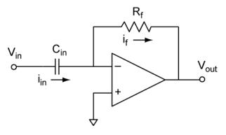
Analysis of the differentiator in the frequency domain is a simple extension of our generalized result for the inverting amplifier.
