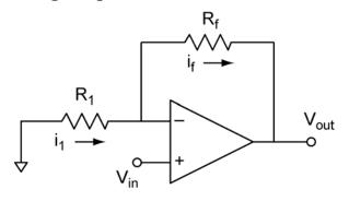
$$\begin{aligned} V_{out} &= \left(1 + \frac{R_f}{R_{in}}\right) V_{in} \\ A_V &= \frac{V_{out}}{V_{in}} = 1 + \frac{R_f}{R_{in}} \\ \frac{\mathrm{d}\,V_{in}}{\mathrm{d}\,I_{in}} &\to \infty \end{aligned}$$
