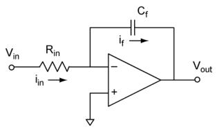
$$\begin{aligned} V_{out} &= -\frac{Z_f}{Z_{in}} V_{in} \\ A_V &= \frac{V_{out}}{V_{in}} = -\frac{Z_f}{Z_{in}} \\ \frac{\mathrm{d}\, V_{in}}{\mathrm{d}\, I_{in}} &= Z_{in} \end{aligned}$$
