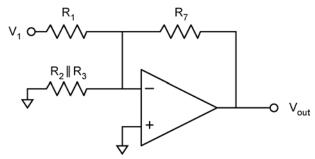
This looks like a summing amplifier with  $V_2 = V_3 = 0$ . The result for the summing amplifier is  $A_{V1} = -\frac{R_7}{R_1}$ . We can do the same analysis for each inverting input. (Why
