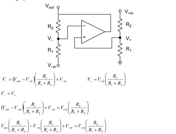
$$V_{out}\!\left(\frac{R_1}{R_1+R_2}\right)\!\!\left(\frac{R_1+R_2}{R_1}\right) = V_{+in}\!\left(\frac{R_2}{R_1+R_2}\right)\!\!\left(\frac{R_1+R_2}{R_1}\right) + V_{-in}\!\left(\frac{R_1}{R_1+R_2}\right)\!\!\left(\frac{R_1+R_2}{R_1}\right) - V_{-in}\!\left(\frac{R_1+R_2}{R_1}\right) = V_{-in}\!\left(\frac{R_1+R_2}{R_1+R_2}\right) + V_{-in}\!\left(\frac{R_1+R_2}{R_1+$$
