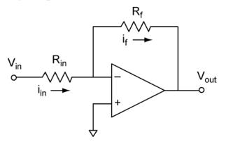
$$\begin{split} V_{out} &= -\frac{R_f}{R_{in}} V_{in} \\ A_V &= \frac{V_{out}}{V_{in}} = -\frac{R_f}{R_{in}} \\ \frac{\mathrm{d}\, V_{in}}{\mathrm{d}\, I_{in}} &= R_{in} \end{split}$$
