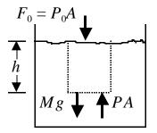
Since there is no acceleration of the liquid at the depth *h*, the forces must balance each other.  $\Sigma F_{\mu} = 0$
