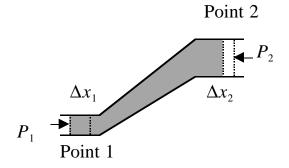
We are going to push a certain amount of fluid up the pipe from point 1 to point 2.  $P_1$  is opposite in direction from  $P_2$  because the rest of the fluid pushes to the left of fluid at point 2 and to the right of the fluid at point 1.
