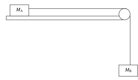
In the first part of this lab, you will be varying the hanging mass ( $M_B$ ) and measuring the force and acceleration of  $M_A$ .
