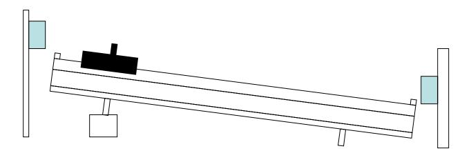
In order to proceed you must measure both the angle and acceleration as accurately as possible for several runs. You measure the angle of the tilt by again measuring the height of the air track above the table at two locations. You should then repeat the experiment at one or more angles.
