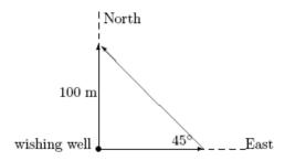
Since north and east are perpendicular to each other, the two strolls and their vector sum form a 45° right triangle. Such a triangle has two equal sides. Hence, the vector to the east has magnitude 100 m. The vector to the northwest is the hypotenuse of the right triangle, and so has magnitude  $\sqrt{(100 \text{ m})^2 + (100 \text{ m})^2} = 141 \text{ m}$ .
