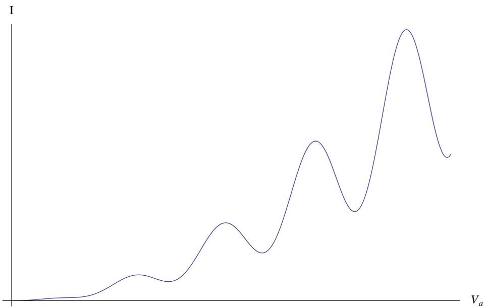
Figure 3.6: The current flowing through the Franck-Hertz chamber as a function of the accelerating voltage. Sharp dips occur at certain critical voltages, corresponding to the energies required to excite the atoms in the gas to higher energy levels.
