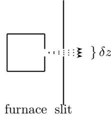
Figure 3.3: Atomic beam emerging from the furnace, collimator arrangement. Note that there is a spread in the  $z$  position of the atoms,  $\delta z$ .
