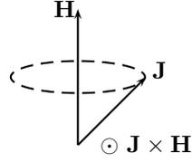
Figure 3.1: If  $\gamma$  is positive, the torque exerted on a magnetic dipole by a fixed magnetic field  $\mathbf{H}$  causes the angular momentum  $\mathbf{J}$  to precess in a clockwise (negative) sense around the direction of  $\mathbf{H}$ , keeping a constant angle with respect to  $\mathbf{H}$ .
