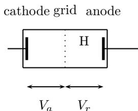
Figure 3.5: A accelerating voltage  $V_a$  accelerated electrons through a chamber containing hydrogen gas. The electrons pass through a grid, following which they experience a small retarding voltage  $V_r$ . The current passing through the chamber is measured as a function of accelerating voltage.
