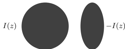
Fig. 5.1. Cross section of two-conductor transmission line. The z direction is out of the page; I(z) flows out of the page, -I(z) flows into the page
