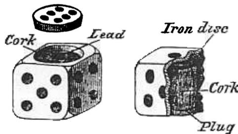
With electric dice, a magnet is switched on to attract the iron disk. Lead and cork maintain the proper weight and balance.
