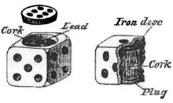
With electric dice, a magnet is switched on to attract the iron disk. Lead and cork maintain the proper weight and balance.
