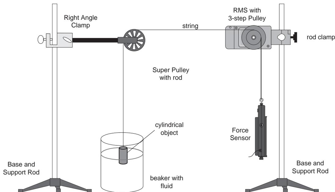
Figure 13.1: Experiment Setup
