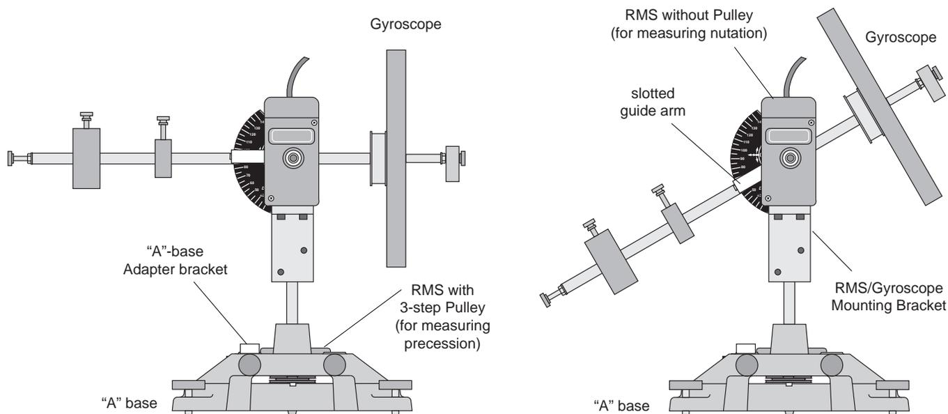
**Figure 12.1: Experiment Setup for Precession and Nutation**
