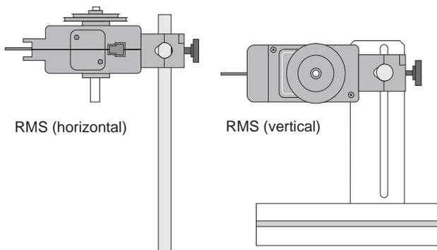
► **NOTE:** When setting up the rotational inertia experiment with the thin rod from the Mini-Rotational Accessory, the Rotary Motion Sensor must be mounted at the top of the support rod so the rod does not interfere with the rotation of the thin rod.
