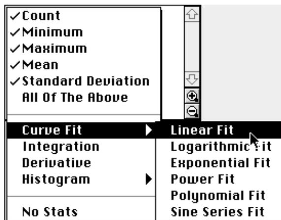
The slope of the linear fit represents the angular acceleration ( $\alpha$ ) and should be entered in Table 1.2.
