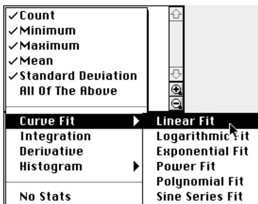
The slope of the linear fit represents the angular acceleration ( $\alpha$ ) and should be entered in Table 2.2.
