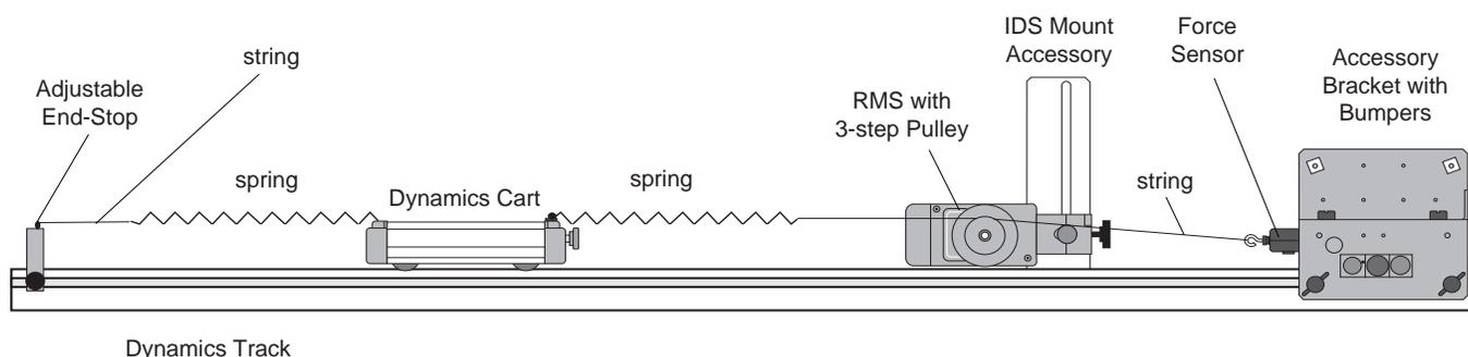
**Figure 8.1: Experiment Setup**
