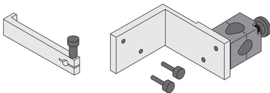
The PASCO ME-8963 RMS/Gyroscope Mounting Bracket attaches the Rotary Motion Sensor to the ME-8960 Gyroscope so the angle of nutation can be detected.
