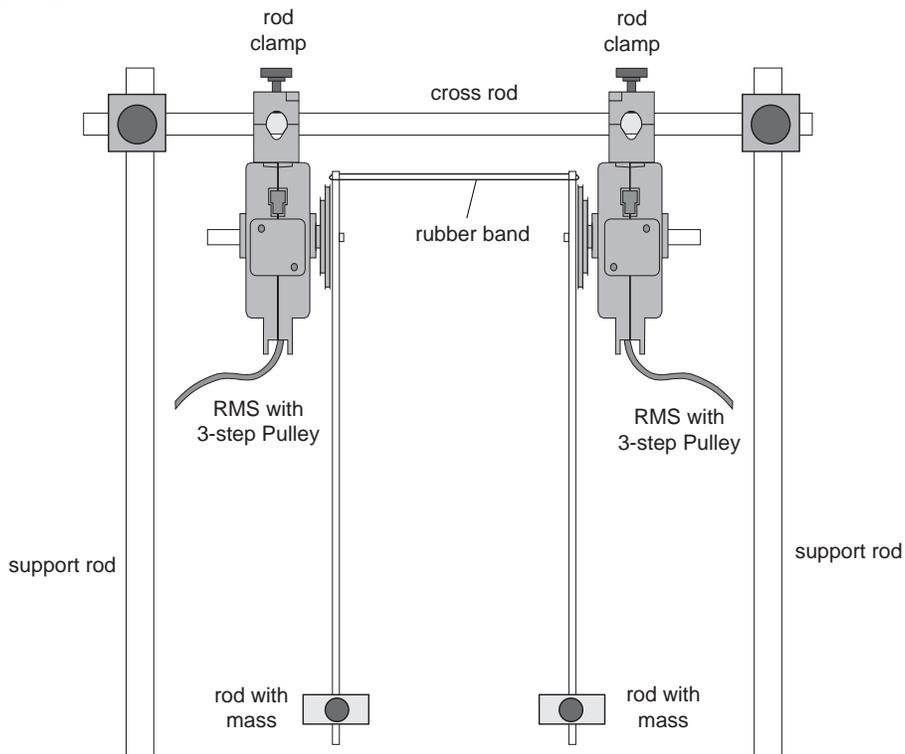
Figure 10.1: Experiment Setup
