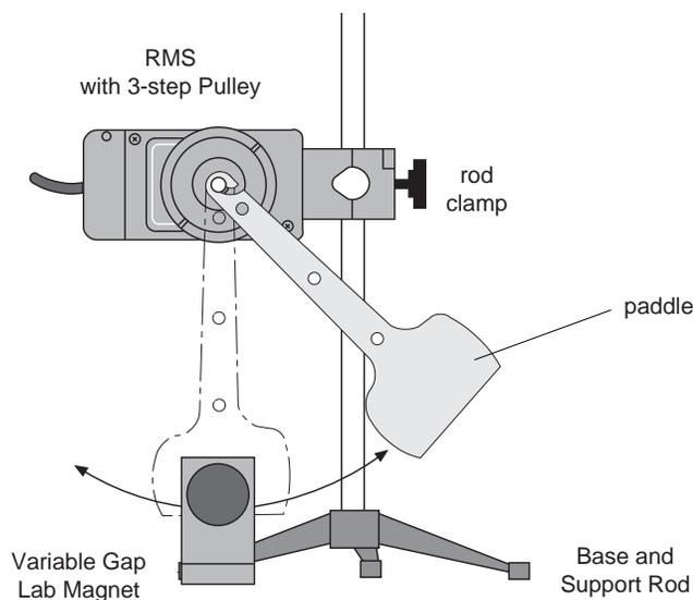
**Figure 18.1: Experiment Setup**
