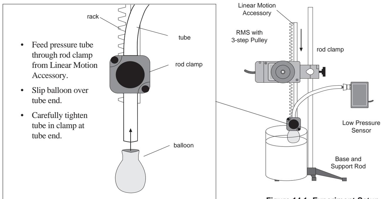
Figure 14.1: Experiment Setup
