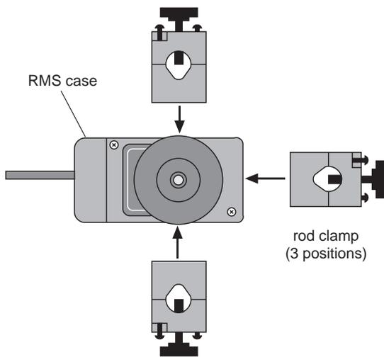
It is possible to mount the RMS horizontally on a support rod, with the 3-step Pulley facing up or vertically, with the pulley facing forward.
