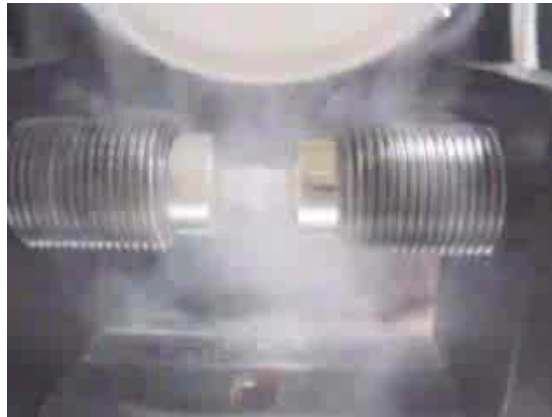
Oxygen disperses as magnets are separated.
