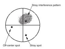
The most common of these are stray interference patterns. These are caused by multiple reflections from the surfaces of the lenses, and may be ignored. If necessary, you may be able to eliminate them by angling the lenses  $1-2^{\circ}$ .
