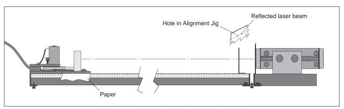
Figure 9: Aligning the Rotating Mirror (M<sub>p</sub>)
