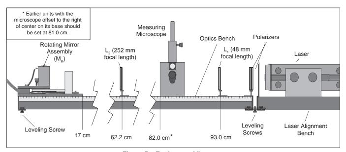
Figure 5: Equipment Alignment
