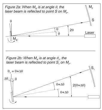
Figure 2 a,b: The Reflection Point on M<sub>E</sub>
