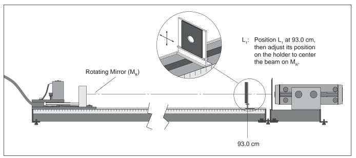
Figure 10: Positioning and Aligning L,
