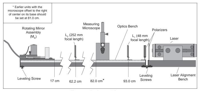
Figure 14: Equipment Alignment
