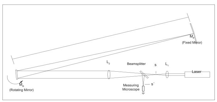
Figure 15: Diagram of the Foucault Method
