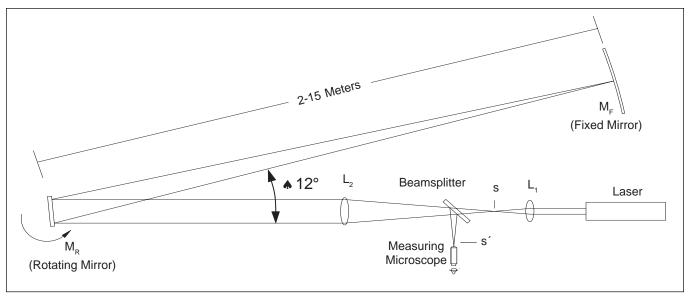
Figure 11: Positioning the Fixed Mirror (M<sub>F</sub>)
