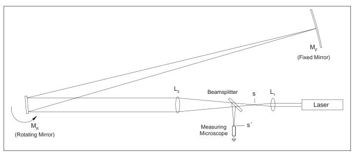
Figure 1: Diagram of the Foucault Method
