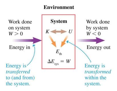
$E_{\mathsf{th}}$  thermal (internal) energy of the system, and W (work) is energy added or removed from the system.
