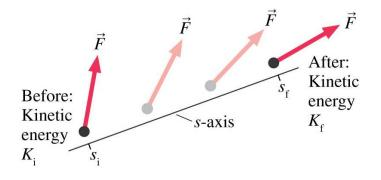
take only the component of the force along the direction of motion
