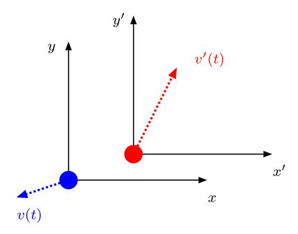
If v(t) or v'(t) are constant, then the primed or unprimed frame is an inertial reference frame
