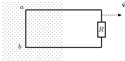
Figure 3: Sketch of a wire loop moving through a magnetic field. The field is normal to the surface of the paper and points into the paper.
