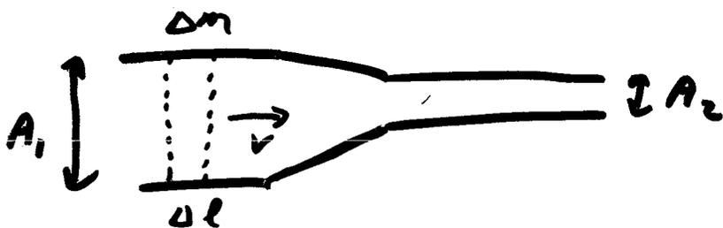
$$\frac{\Delta m}{\Delta t} = \rho \frac{\Delta V}{\Delta t} = \rho A \frac{\Delta l}{\Delta t} = \rho A v$$
