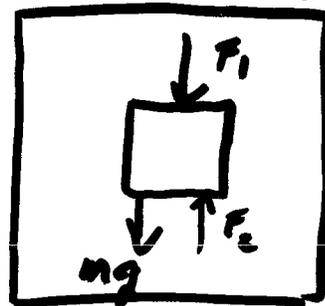
$$\begin{aligned}\sum F_y &= F_2 - F_1 - mg \\ &= P_2 A - P_1 A - mg \\ &= \rho g h_2 A - \rho g h_1 A - mg \\ &= \rho g A (h_2 - h_1) - mg \\ &= \rho g V - mg \\ &= \underset{\substack{\uparrow \\ F_B}}{m_f g} - mg\end{aligned}$$
