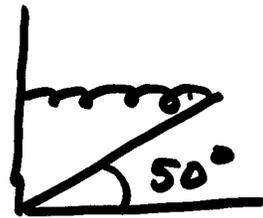
$$\Sigma \tau = 0 \quad + F \left( \frac{L}{2} \right) \sin 50^\circ - mg \left( \frac{L}{2} \right) \sin 40^\circ = 0$$
