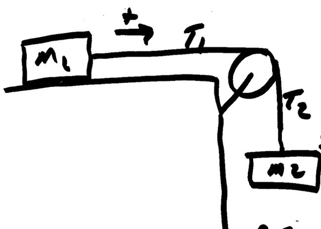
Pulley has moment of inertia  $I$
