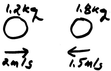
$$\begin{aligned}m_1 &= 1.2 \text{ kg} \\m_2 &= 1.8 \text{ kg} \\v_{1i} &= 2.0 \text{ m/s} \\v_{2i} &= -1.5 \text{ m/s} \\v_{1f} &=? \\v_{2f} &=?\end{aligned}$$
