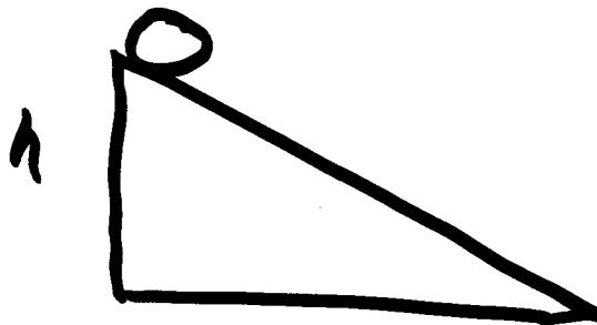
$$mgh = \frac{1}{2}mv^2 + \frac{1}{2}I\omega^2 \quad v = \omega r$$
