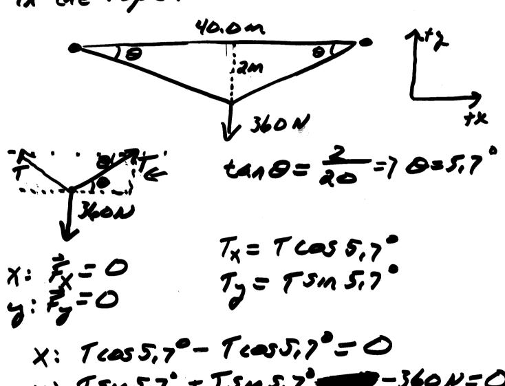
X:  $T \cos 5.7^{\circ} - T \cos 5.7^{\circ} = 0$ y:  $T \sin 5.7^{\circ} + T \sin 5.7^{\circ} = 360 N = 0$  $T = \frac{360 N}{25 m 5.7^{\circ}} = \frac{1810 N}{180 N}$
