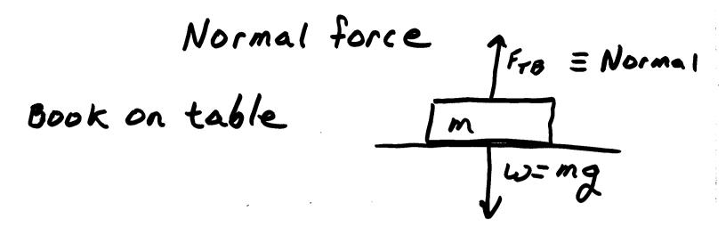
Normal force always perpendicular to contact surface
