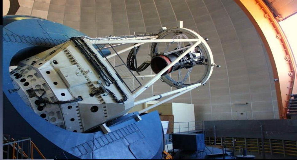
The 520 megapixel Dark Energy Camera (DECam)
