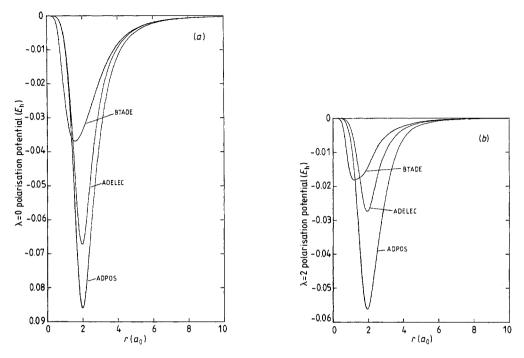
**Figure 1.** (a) Spherical ( $\lambda = 0$ ) and (b) non-spherical ( $\lambda = 2$ ) radial expansion coefficients (see equation (9)) of the three polarisation potentials discussed in § 2.3: the adiabatic electron-H<sub>2</sub> potential (ADELEC), the adiabatic positron-H<sub>2</sub> potential (ADPOS) and the non-adiabatic electron-H<sub>2</sub> potential (BTADE). The ADELEC and ADPOS potentials were cut off using equation (6) with  $r_c = 1.5a_0$ .
