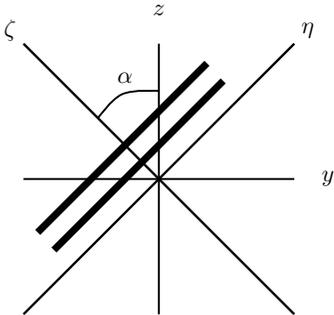
FIG. 1: Relation between two Cartesian coordinate frames: One attached to the earth  $(x, y, z)$ , where  $-z$  is the direction of gravity, and one attached to the parallel-plate Casimir apparatus  $(\zeta, \eta, \chi)$ , where  $\zeta$  is in the direction normal to the plates. The parallel plates are indicated by the heavy lines parallel to the  $\eta$  axis. The  $x = \chi$  axis is perpendicular to the page.
